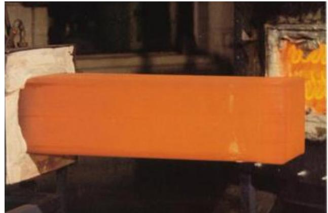
This horizontal electrically fired 230® retort replaced an alloy 600 retort which lasted only an average of eight months in 1400 to 2200°F (760 to 1205°C) service in hydrogen atmosphere. The 230 retort was still in excellent condition after 24 months service, as shown.
